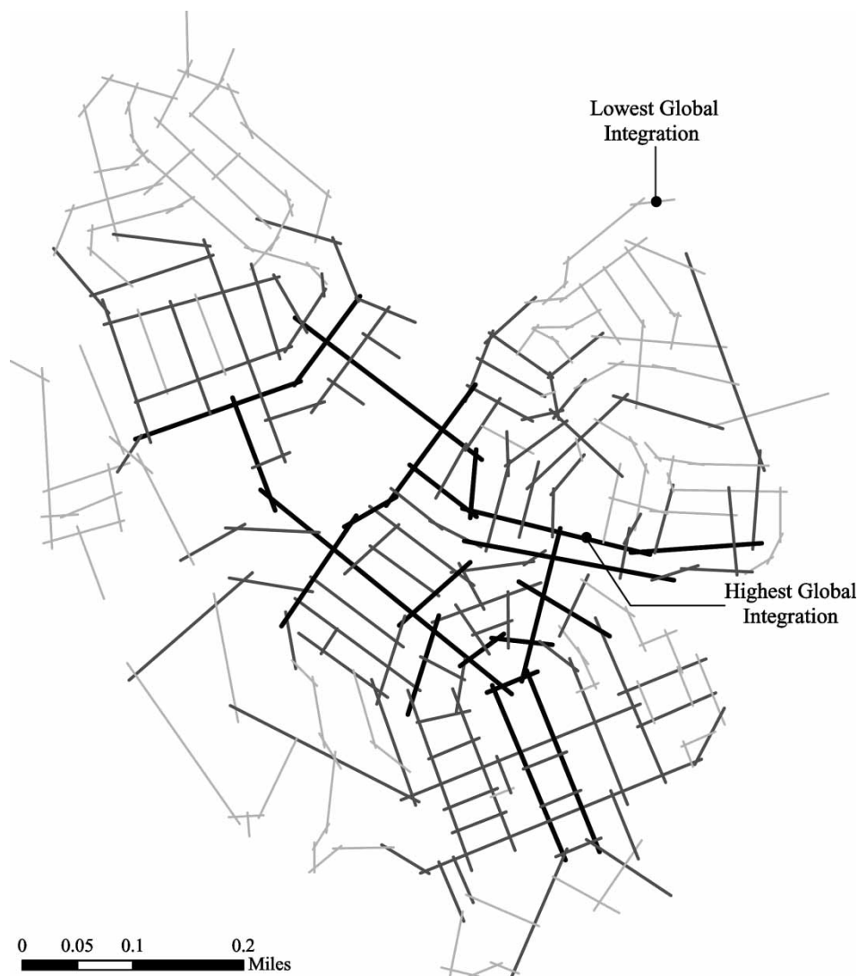
Figure 3. Axial map of the pedestrian network for the New Urbanist neighbourhood; the 10% global integration core shown in heavy black and the 50% globally most segregated lines shown in light grey.
